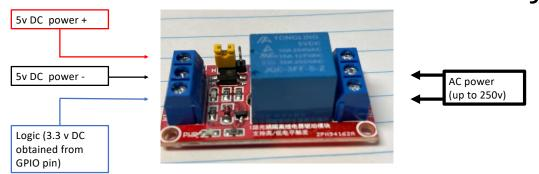
A relay is a switch that can be "flipped" electronically.
